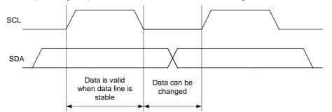
\* Note with caution that if the SDA data is changed while the SCL line is at high level, it will be treated as a START, RESTART, or STOP condition.
